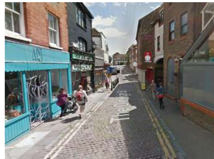
↑ Bayle Street: design treatment suggests pedestrian-priority space however cobbles are uneven, narrow footways on both sides, bollards and columns obstruct pedestrian movement, variable quality of materials
