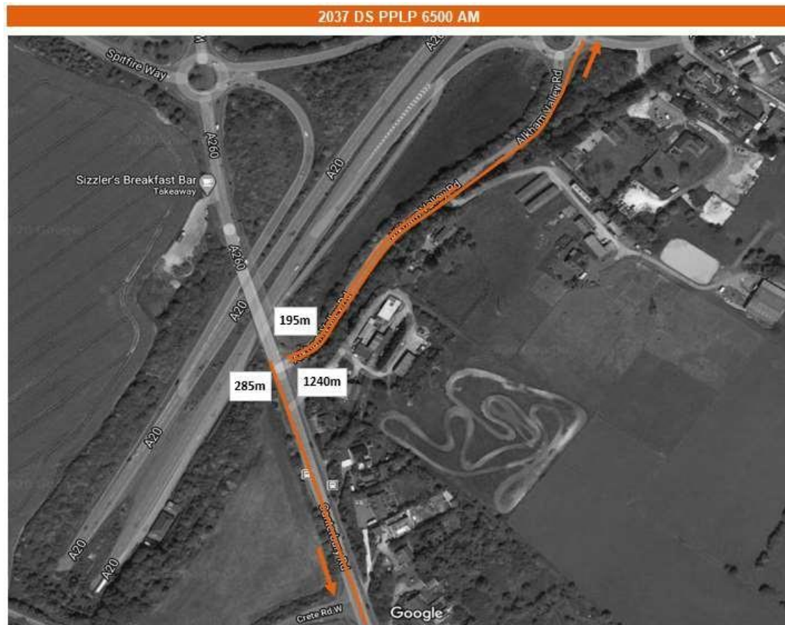
Image 6 – Canterbury Rd-A260 Alkham Valley Rd – 2037 Queue Length Comparison of the DM and DS Scenarios
