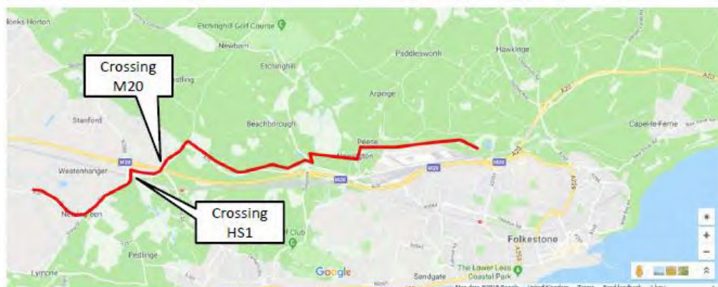
Approximately 11km of 560mm OD (494mm ID) main. Total implementation period from the start of planning through to construction completion is 4-5 years to allow for the two crossings of strategic infrastructure.
