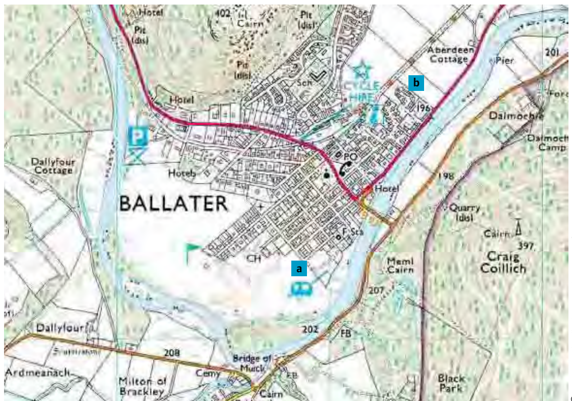
Figure 3.8 Ballater, Aberdeenshire – the ability for future growth is not compromised in the south-west of the village (a) with its permeable street pattern, but more recent cul-se-sac type development in the north-east (b) does not allow for a connected growth of the village.
