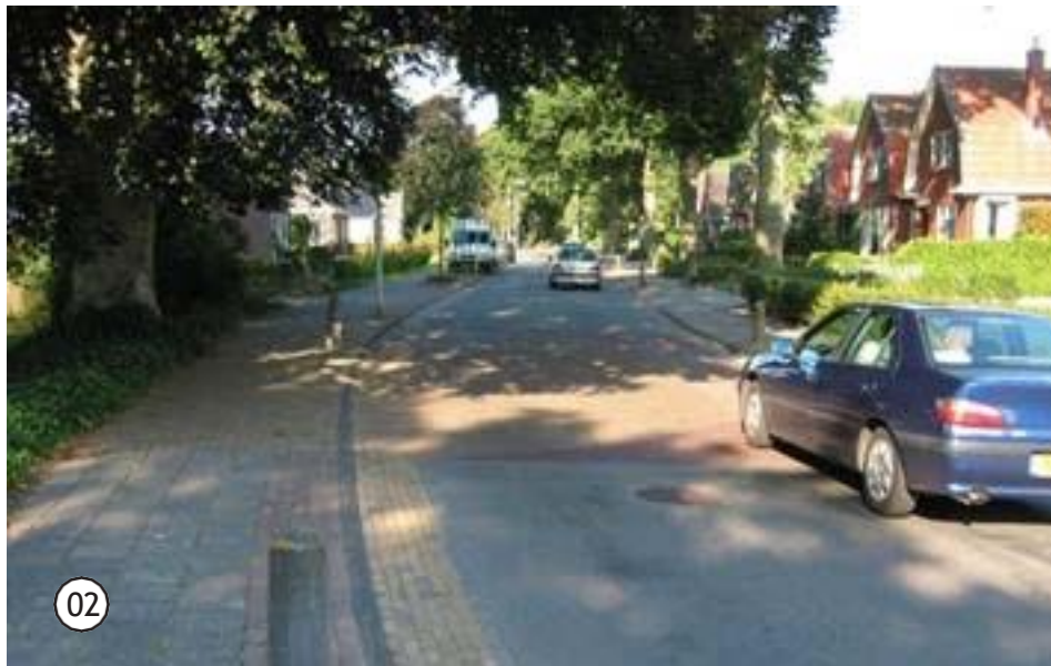
01,02. The deliberate use of ambiguity, through the removal of signs and road markings, has actually led to a reduction in casualty figures in parts of Holland, Denmark and Sweden.
