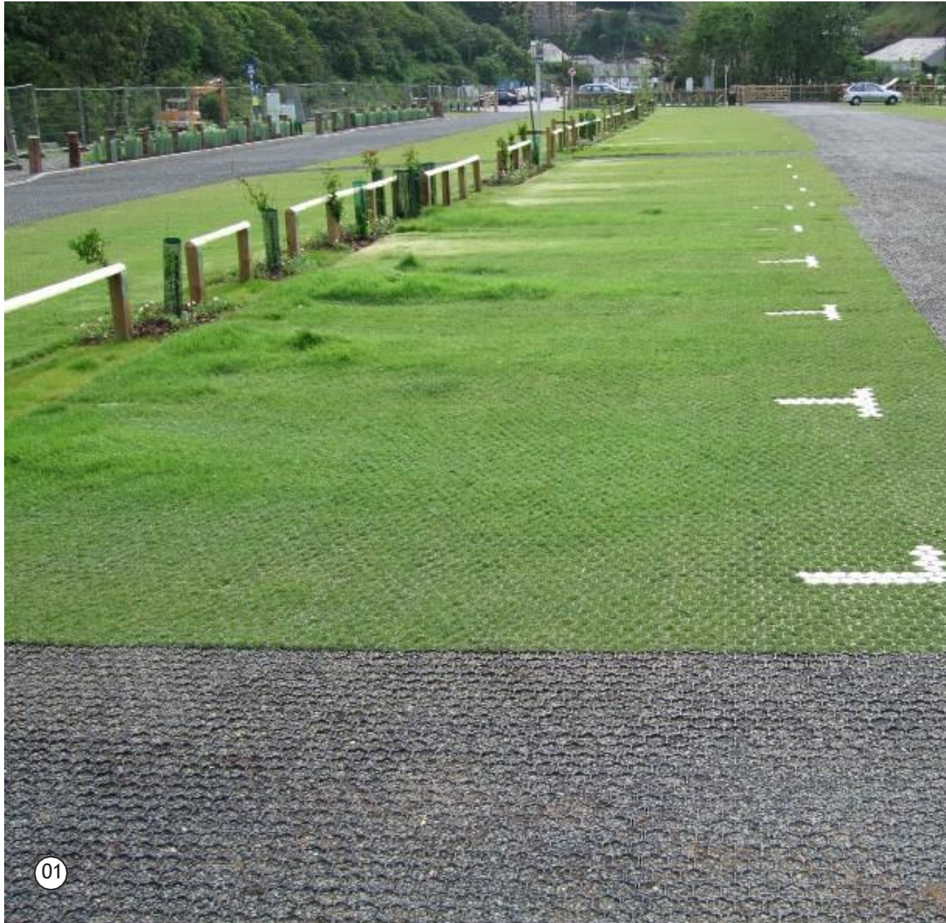
01 - 03. The use of grasscrete, sometimes with synthetic materials, can reduce the visual impact of car parking
