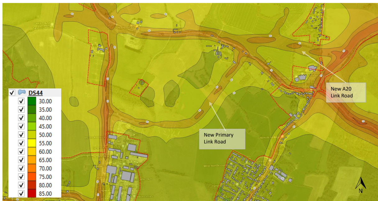
Image 13-2 Noise Contours showing absolute noise level contours attributable to new A20 and Primary Road Link for 2044
