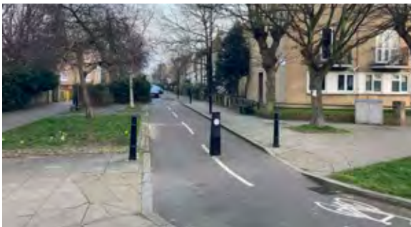
Fig. 5.26: Tertiary street precedents, including filtered permeability (below), with segregated footpaths from the carriageway alongside landscaping
