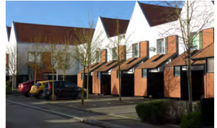
Fig. 5.55: Parking in front of the dwellings is interspersed with tree planting to soften its impact
