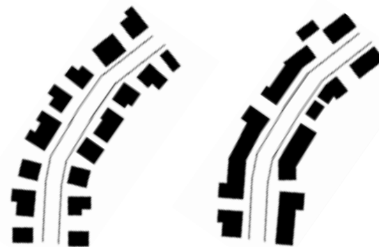
Fig. 5.46: Continuous frontages (right) provide a strong sense of enclosure (right) compared to predominantly detached dwellings (left). Depending on the intended character of the area, either may be appropriate in the right location.
