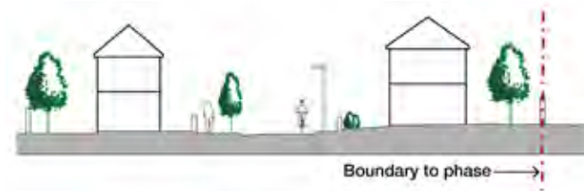
Fig. 5.50: Where possible, locate boundaries to phases along the line of the rear of building plots to minimise the potentially disjointed appearance between different building phases.
