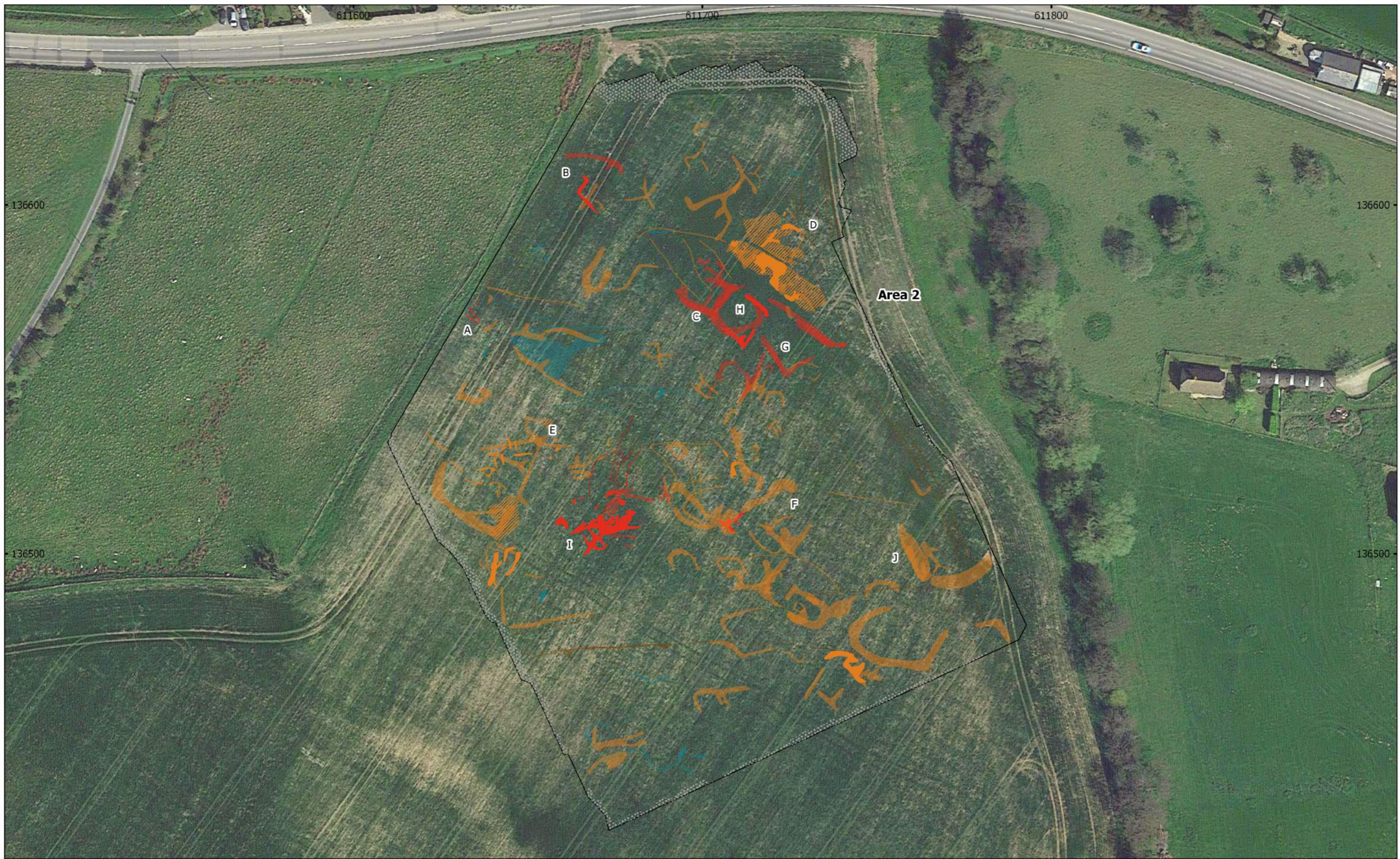
MSTR375 - Ground Penetrating Radar and Magnetometry Survey of the Roman Villa at Otterpool, near Hythe, Kent Figure 10 - GPR Combined Interpretation Over Satellite Imagery 1:1,000 @ A3 Copyright Magnitude Surveys Ltd 2018 Contains satellite imagery © Google 2018
