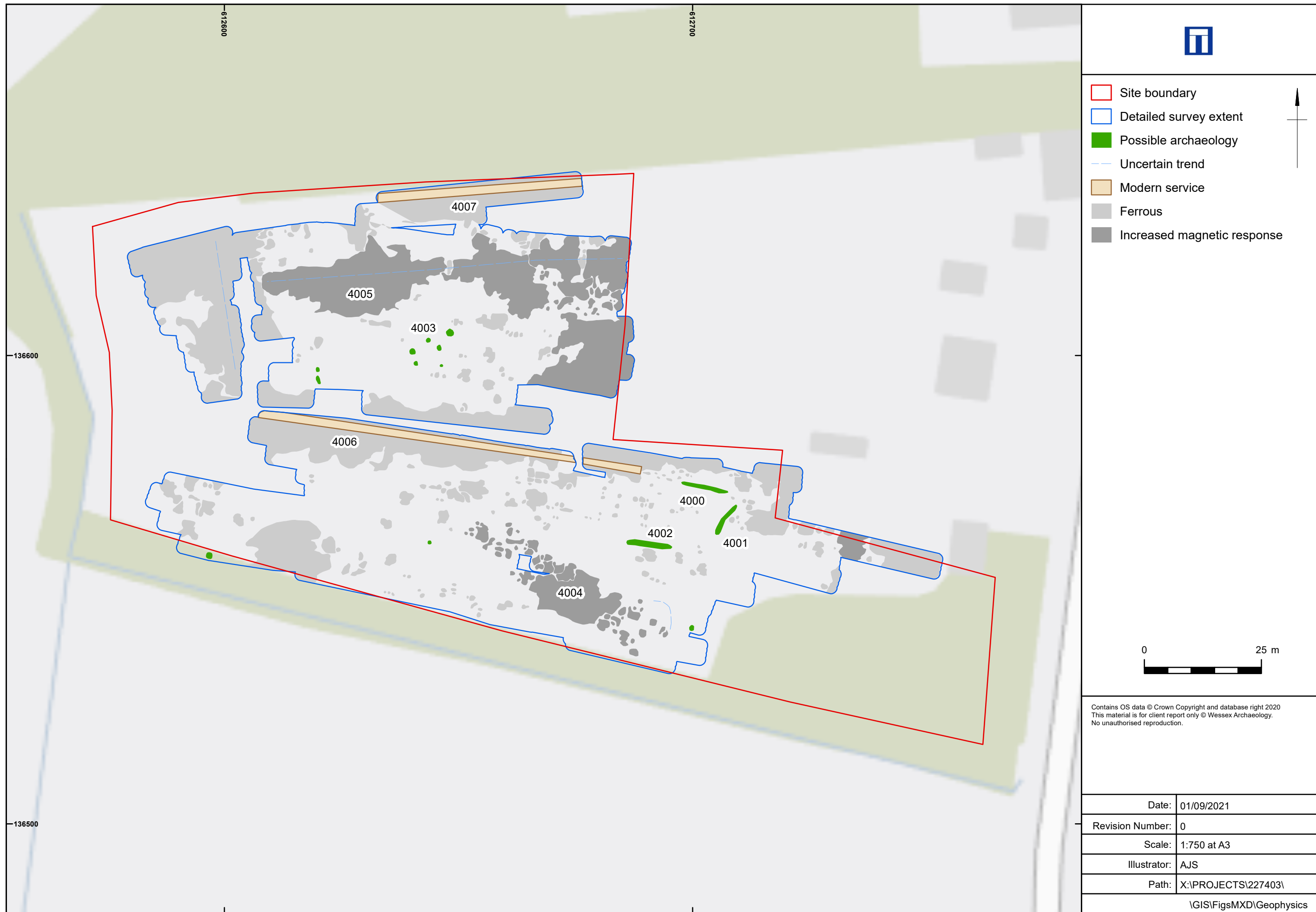
Detailed gradiometer survey result: interpretation
