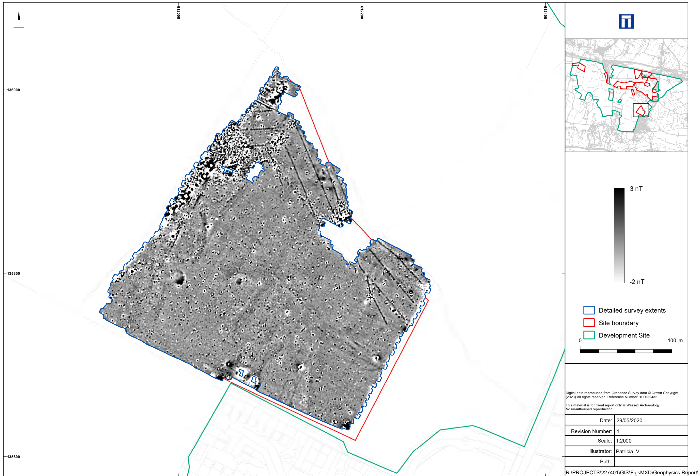
Detailed gradiometer survey results: Greyscale plot Area 5
