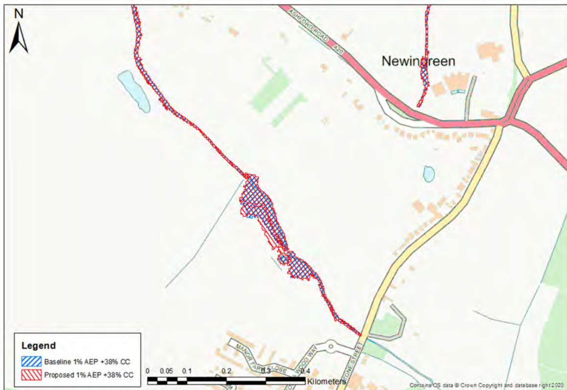
Figure 3-6 Comparison of baseline and proposed flood extents for the 1% AEP +38% CC at the upstream end of North Lympne Drain
