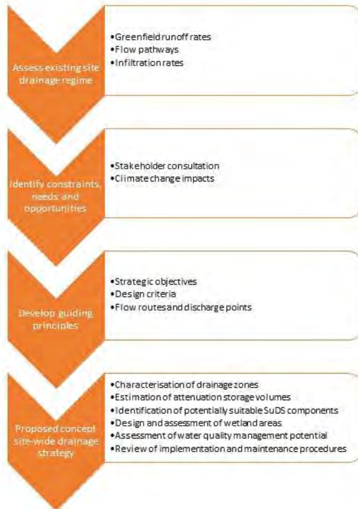
Figure 12: Development of the surface water drainage strategy
