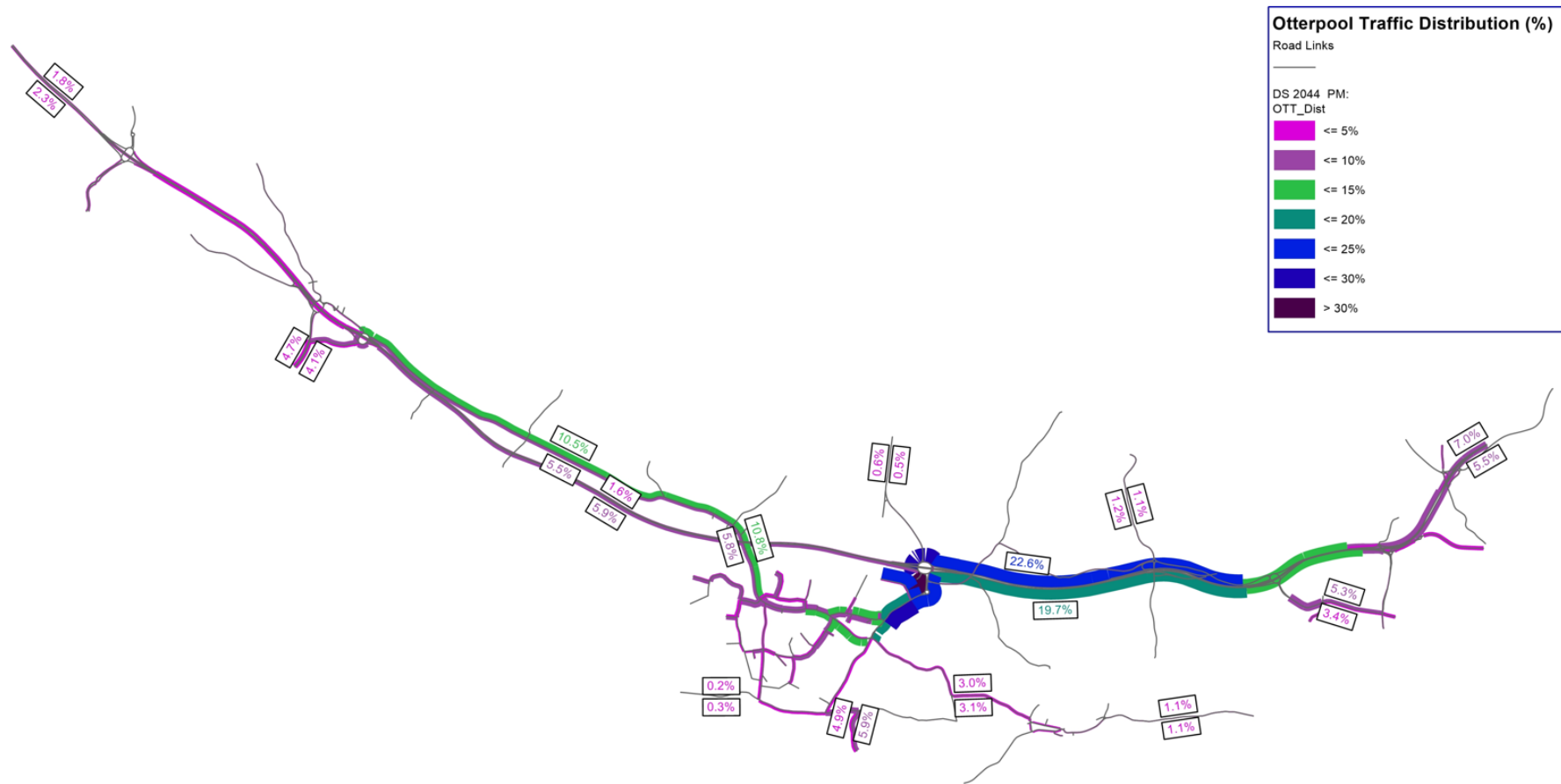
Figure 17 Otterpool Traffic Distribution on the Wider Highway Network – PM Peak (2044 8.5k)
