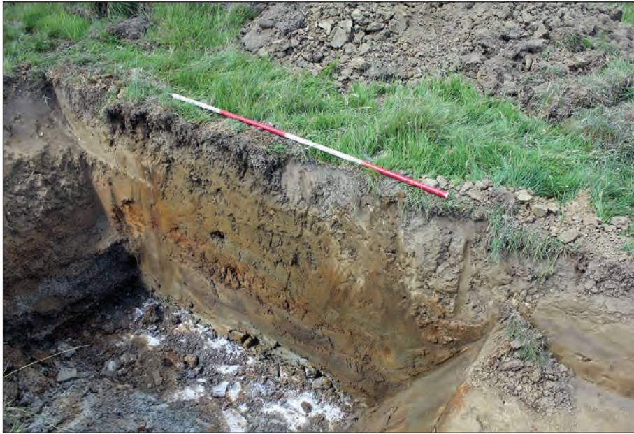
Plate 1: Test Pit 3 – Minerogenic alluvium and colluvial clay overlying Hythe Formation.
