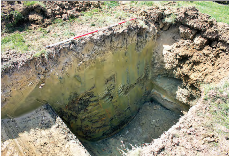
Plate 2: Test Pit 2 – Gravelly clay and colluvial clay overlying Sandgate Formation.
