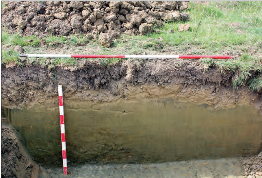
Plate 4: Test Pit 1 – Colluvial clay overlying Sandgate Formation.
