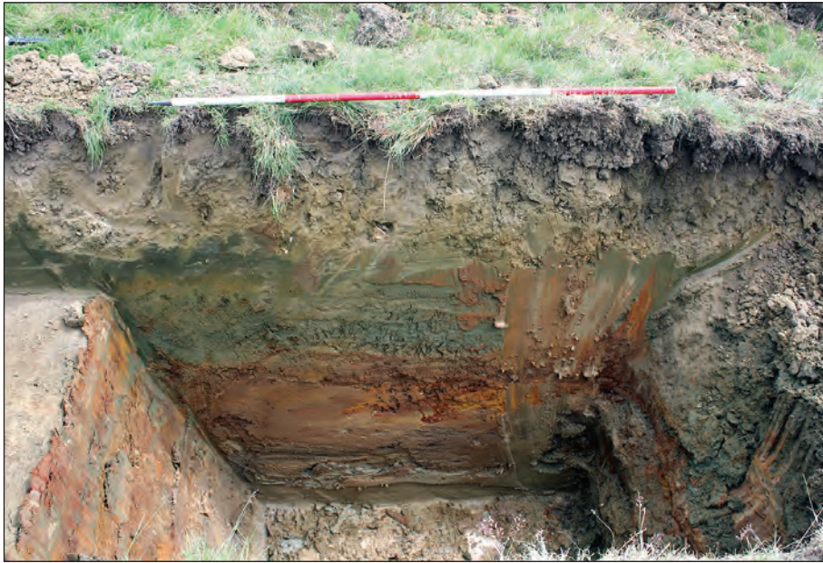
Plate 3: Test Pit 4 – Minerogetic alluvium and colluvial clay overlying Hythe Formation.
