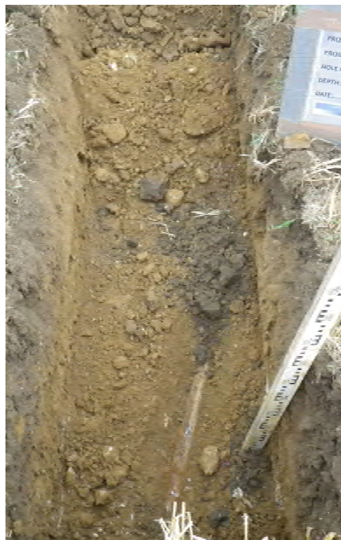
[TRIAL PIT NUMBER 219: METAL PIPE]
