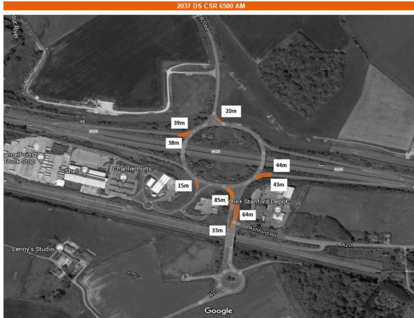
Image 9 – M20 Junction 11 Initial Mitigation 2037 Queue Length
