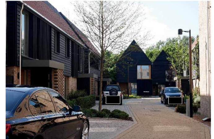
Fig. 5.21: A residential home zone integrates non-allocated parking along the street within a shared surface space
